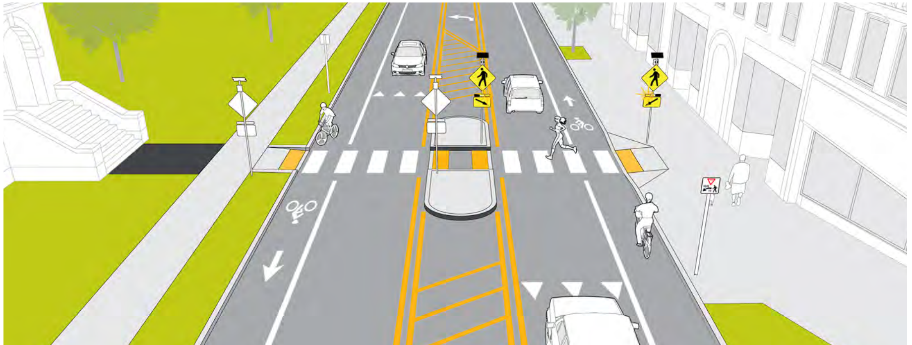
Figure 5.2 Enhanced Pedestrian Crossing Treatments
