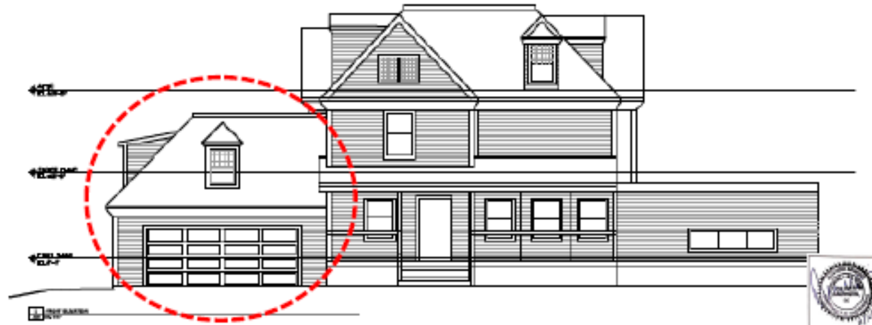
Proposed front elevation (new garage/addition indicated)
