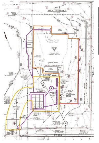
Stormwater Management includes: one catch basin, one manhole, trench drains and 12 infiltration galleys.
