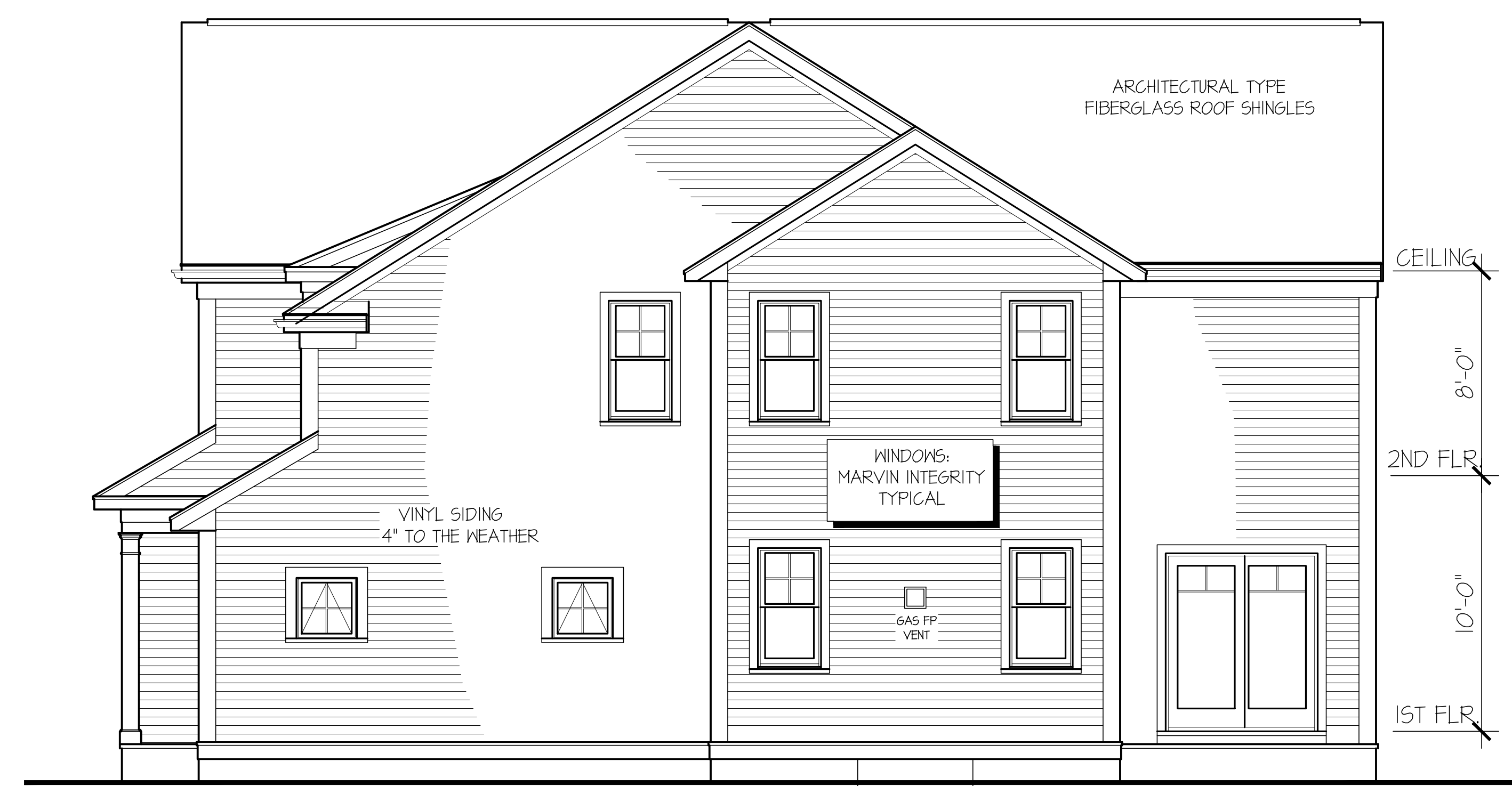
C RIGHT SIDE ELEVATION 1/4" = 1'
