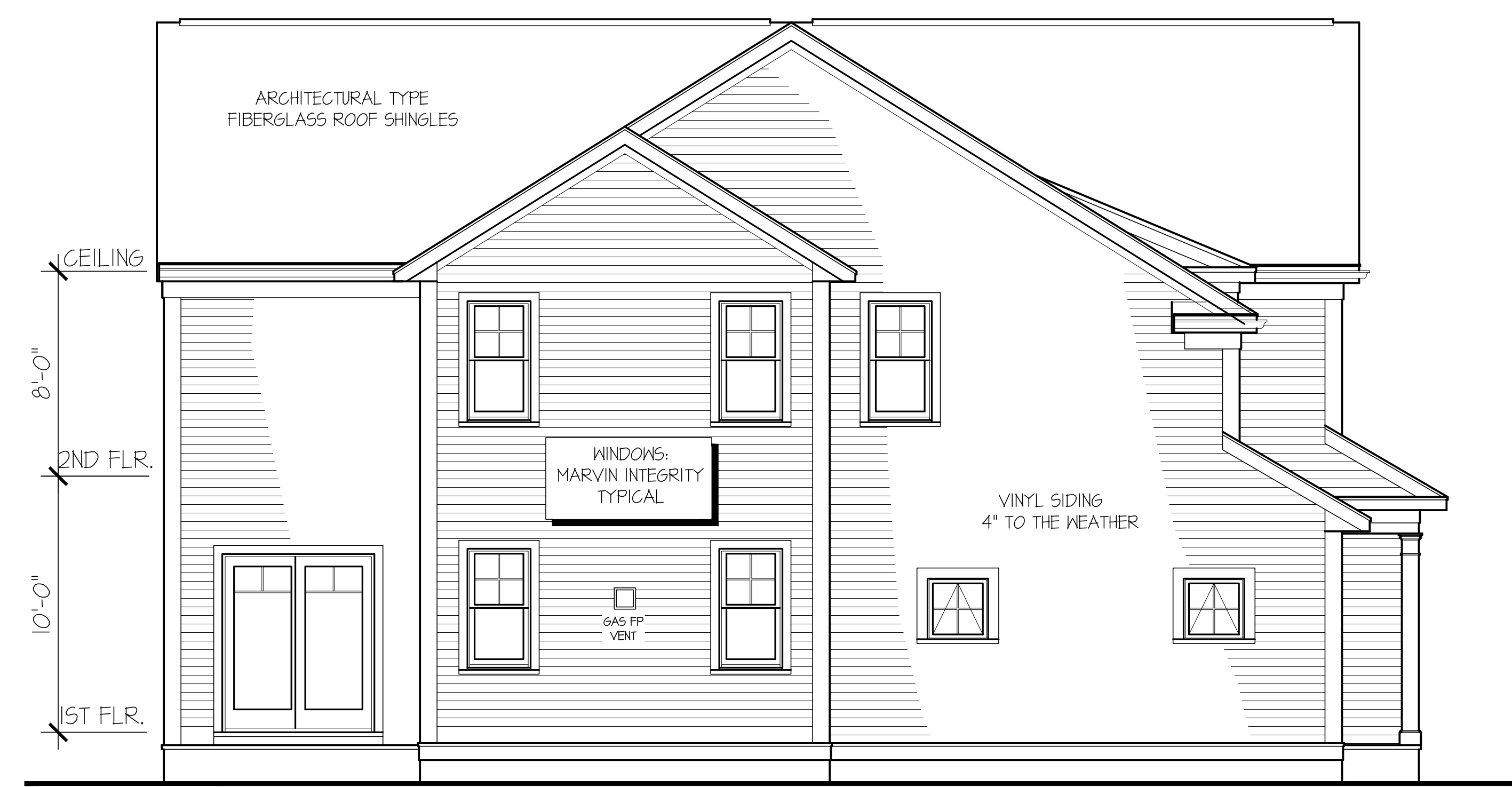
B LEFT SIDE ELEVATION 1/4" = 1'
