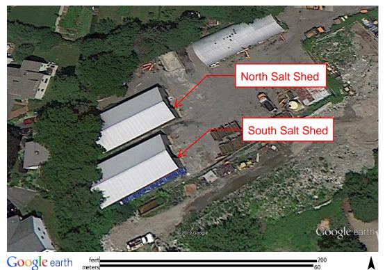
Ariel view of salt sheds at Newton DPW Crafts Street location. Both sheds appear to be constructed around same time and are same size at 40'x84' and house approximately 1,000 cubic yards of road salt. Both buildings have been labeled as Unsafe Structures by the Inspectional Services Department on 10-31-12
