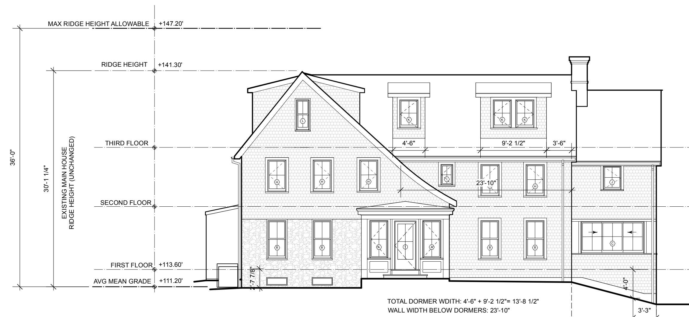
PROPOSED MAIN HOUSE FRONT ELEVATION Scale: 1/8" = 1'-0"
