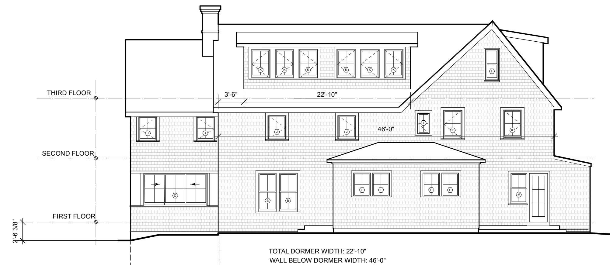
PROPOSED MAIN HOUSE REAR ELEVATION Scale: 1/8" = 1'-0"
