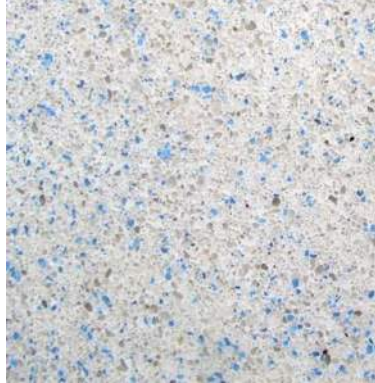
Aggregate Pool Plaster
