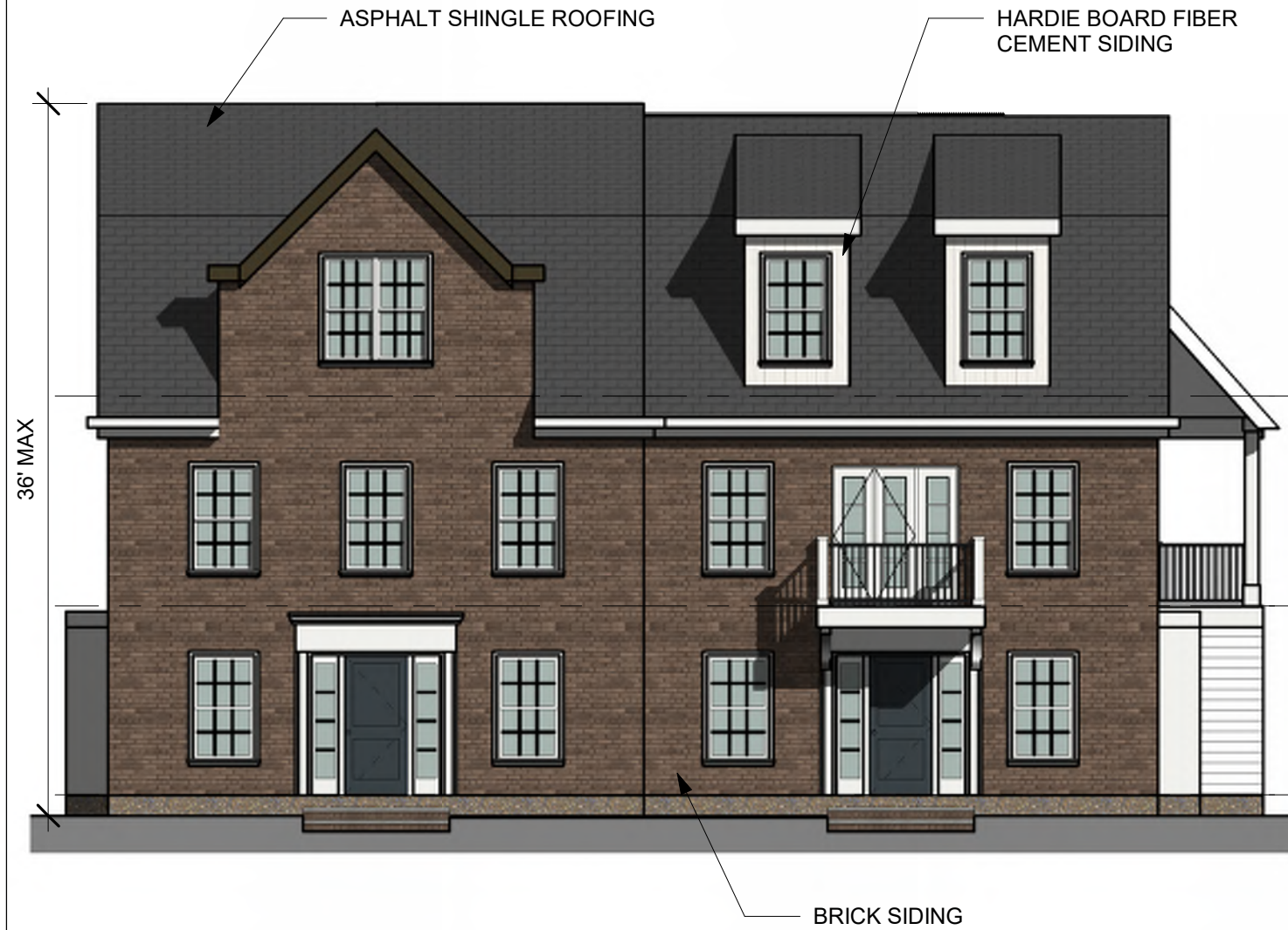
1 BUILDING 1 FRONT ELEVATION 1/8" = 1'-0"
