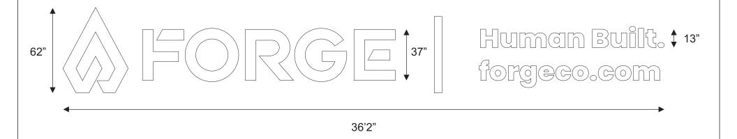
Internally illuminated (LED) channel letters. Aluminum edges and backs, white translucent acrylic faces mounted to raceway that is painted to closely match the building color.
