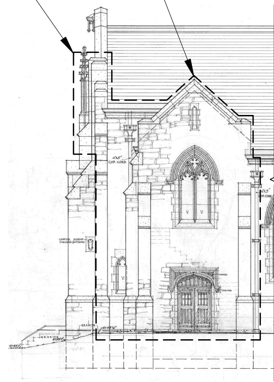
3 WEST END SOUTH ELEVATION ALTERNATE #1 R-4 1/16" = 1'-0"
