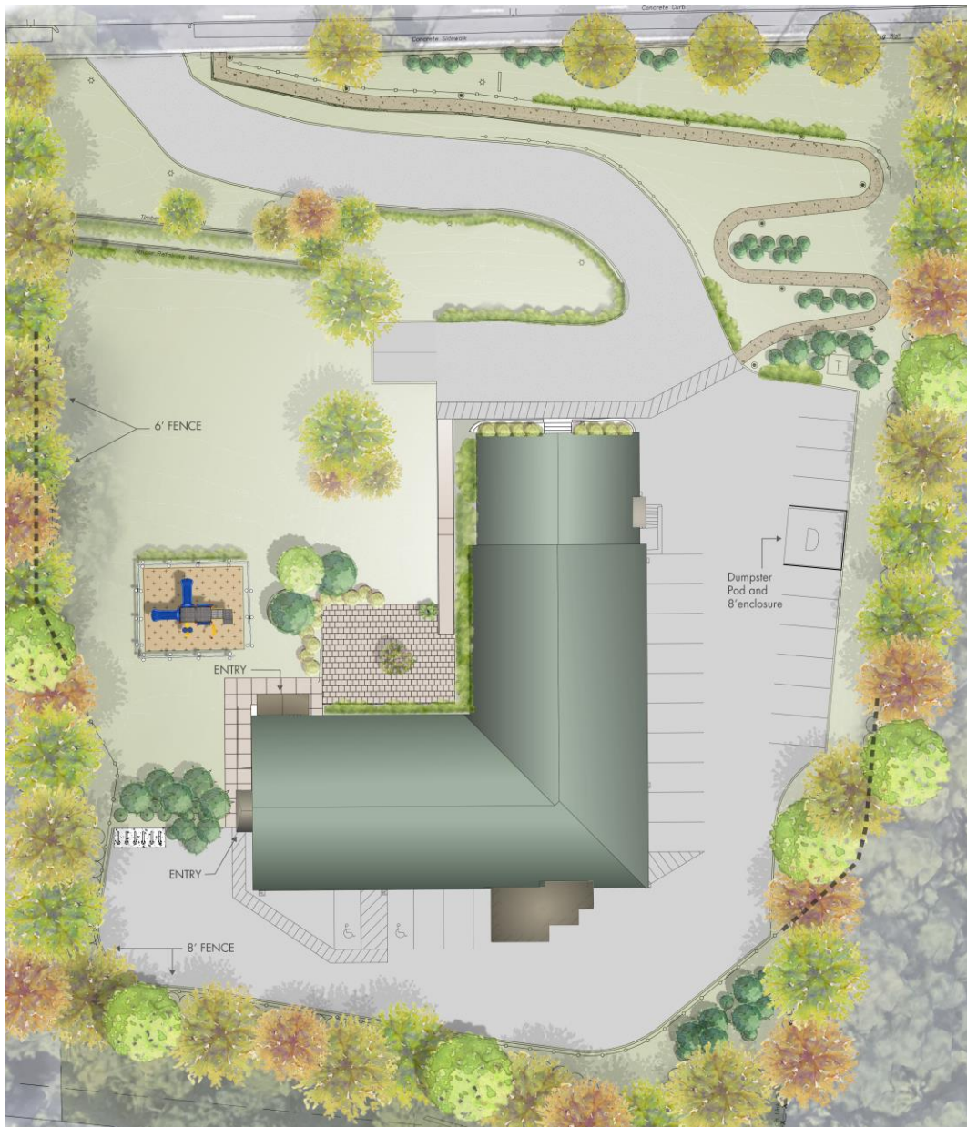
Aerial view with proposed improvements: ADA walkway, playground, plaza, privacy fencing and privet, drainage, dumpster re-siting, landscaping
