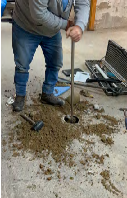
Engineer digs test pit at 112 Grasmere
