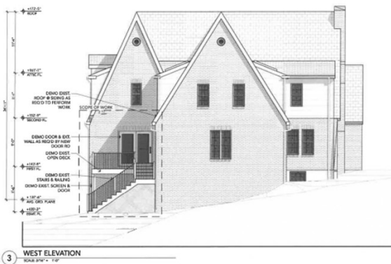
Existing West Elevation
