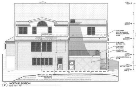
Existing North Elevation
