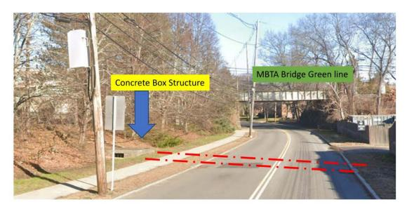
There are two 24" reinforced concrete pipes (see following photo) that cross underneath Grove Street which transmits Runaway Brook from the golf course right side of the photo (behind the fence) to the concrete box structure shown on the right side of Grove Street. The pipe are relatively shallow The contractor of record needs to be made aware of this. This crossing is not shown on the submitted plan.
