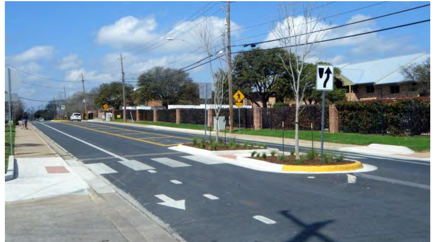
Example: Staged crosswalk with refuge island
