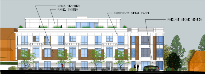
NORTH ELEVATION— BEACON STREET FACADE
