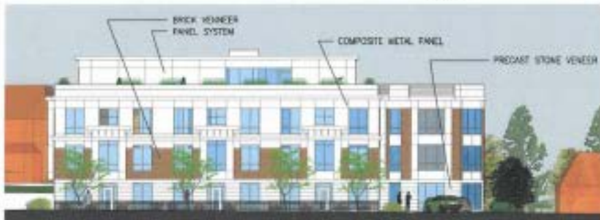
NORTH ELEVATION - BEACON STREET FACADE
