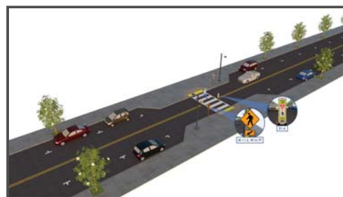
The enhancements shown in this rendering of a midblock crosswalk include high-visibility markings, curb extensions, in-street pedestrian crossing signs, lighting, and warning signs. Federal Highway Administration.
