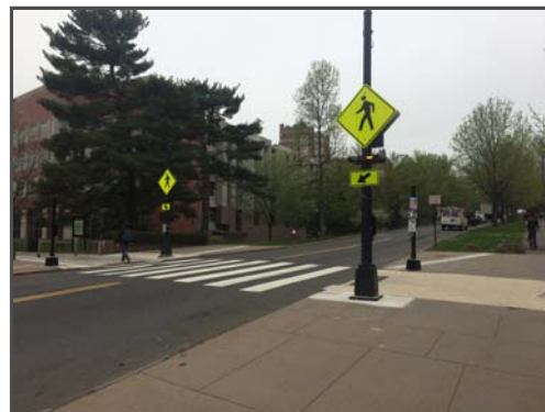
A Rectangular Rapid-Flashing Beacon (RRFB) in Princeton, New Jersey. Federal Highway Administration.
