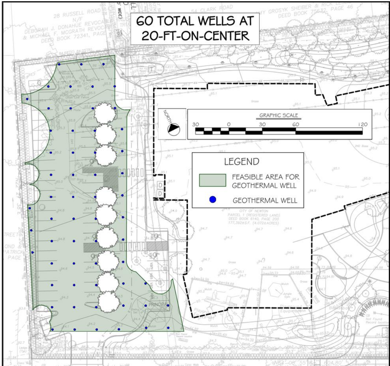
Figure 4. Possible wellfield layout in the western parking area at 20-feet-on-center.
