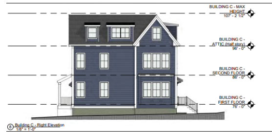
Building C - Right Elevation 1/8" = 1'-0"
