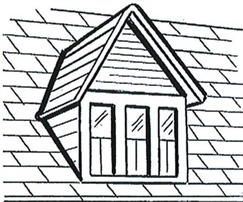
Fig. 1: Sketch of a typical dormer
