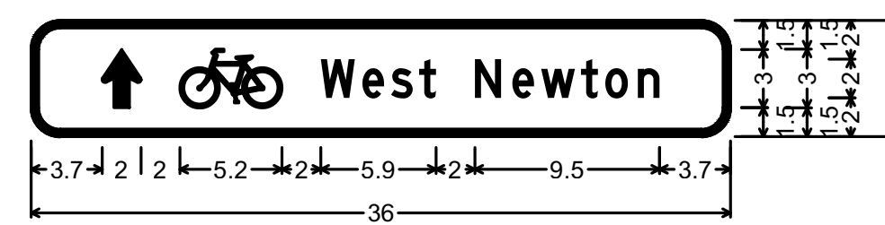
D1-1B: 1.5" Radius, 0.4" Border, White on, Green; Standard Arrow Custom 3.0" X 2.0" 90'; Bicycle; "West Newton", D;
