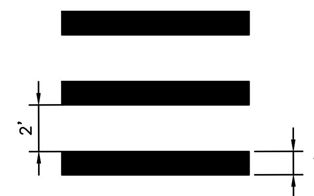
CROSSWALK MARKING IN BICYCLE LANE
