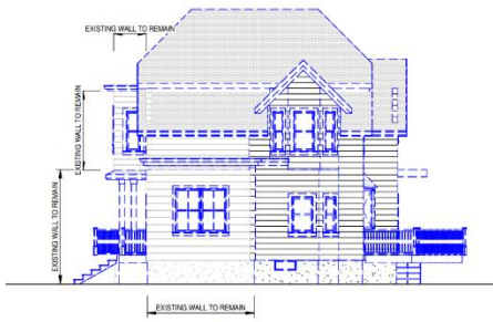
8 Right Elevation - Demolition 1/8" = 1'-0"
