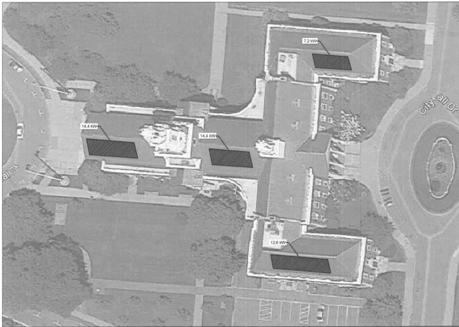
Newton City Hall - 48.6KW Roofmount System
