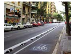
Bike Lane with Raised Separation
