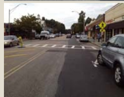
FIGURE 9-4. Pedestrian sight distance and parking restriction needed for parallel parking.
