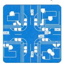
reducing speeds at intersections with substantial pedestrian activity and improve the realm of the pedestrian. They reduce speeds for right-turning vehicles while allowing unimpeded left turning movements. They can also be used to delineate onstreet parking spaces, but may result in the loss of the parking space adjacent to the intersection. Also, they may force bicyclists to merge into the traffic lane at an intersection.
