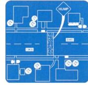
2) Speed tables: Speed tables are flat-topped speed humps that are often constructed of brick or other textured materials on their flat section. On a speed table, the ramps are often more gently sloped than on a speed hump, and the entire wheel-base of the
