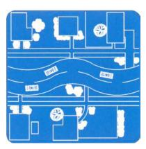
to another. By causing traffic to deviate on the otherwise straight roadway, chicanes reduce vehicular speeds. In contrast to speed humps, they do not cause increased noise and are relatively easy to maneuver by trucks. However, they must be designed so that drivers do not cross the center-line, and curb realignment can be costly. A loss of onstreet parking may also result.
