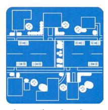
2) Median barriers: These are islands in the middle of a street than continue through an intersection, preventing through movement of vehicles that would otherwise cross the road. They can improve safety by preventing dangerous turning movements and reduce cut-through traffic where it is desired. However, they also limit access for local
