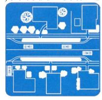
location that narrows the road while maintaining the straight-away. They result in a loss of on-street parking, but can reduce vehicle speeds and lead to lower traffic volumes. Chokers can be easily negotiated by large vehicles and trucks, since the travel lane is not reduced in width. However, a choker may force bicyclists to merge into traffic.
