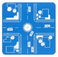
improving safety in areas where large traffic volumes are not expected. However, they can be difficult for large vehicles to navigate and may require additional maintenance, such as landscaping. Also, they may cause cars to encroach on the adjacent sidewalk at intersections and may result in a loss of on-street parking.
