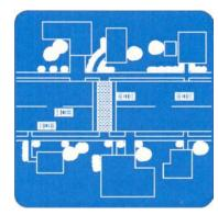
Results: The same as for speed tables – an 18% decrease in speeds (36.7 mph to 30.1 mph) and a 45% decrease in accidents (6.7 to 3.7 per year). Again, this is for a 22-foot speed table, which is similar to a raised crosswalk.
