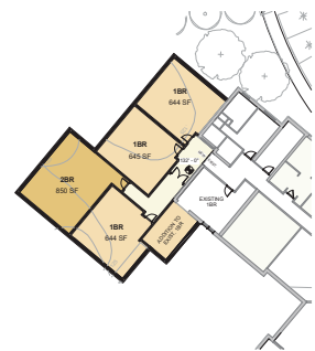
LVL 1 (132'-0") - LOWER ADDITION SCALE: 1/16" = 1'-0" 3,940 Gross SF
