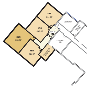
LVL 0 (123'-8") - LOWER ADDITION SCALE: 1/16" = 1'-0" 3,840 Gross SF
