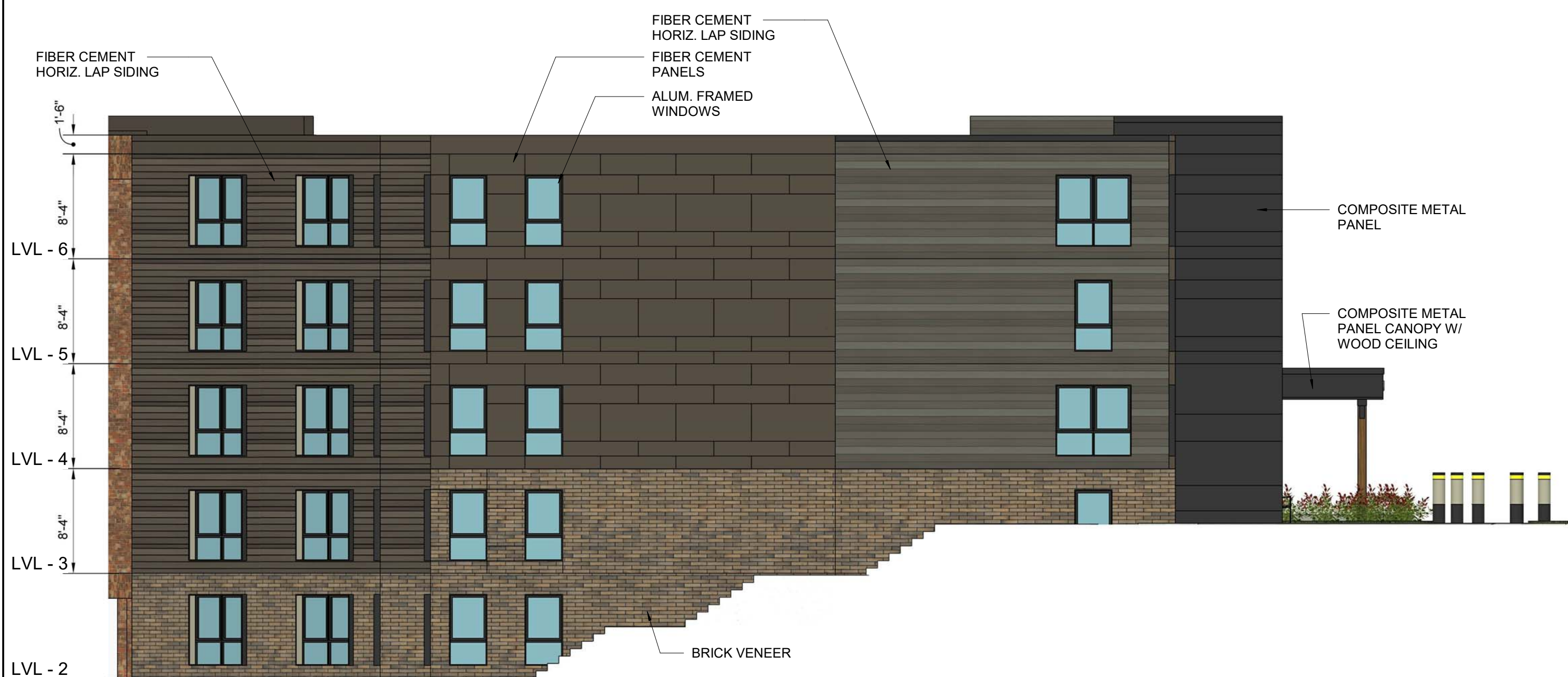
4 - UPPER - SOUTH ELEVATION SCALE: 1/8" = 1'-0"
