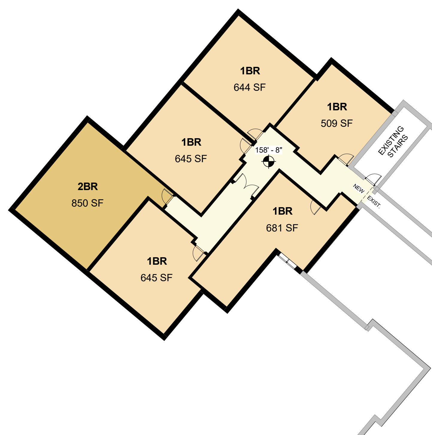
LVL 4 (158'-8") - LOWER ADDITION SCALE: 1/16" = 1'-0"
