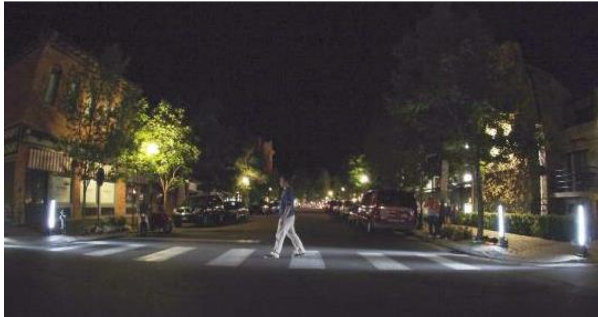
POST LIGHTS REFERENCE AND ILLUMINATE PEDESTRIAN CROSSWALKS
