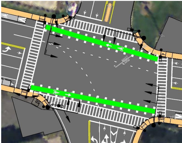
Signalized Separated bike lane
