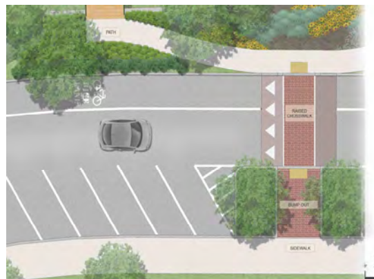
The plan image identifies suggested roadway treatments aimed at slowing traffic and improving pedestrian and bicyclist accommodations, including the bump outs and raised crosswalks.
