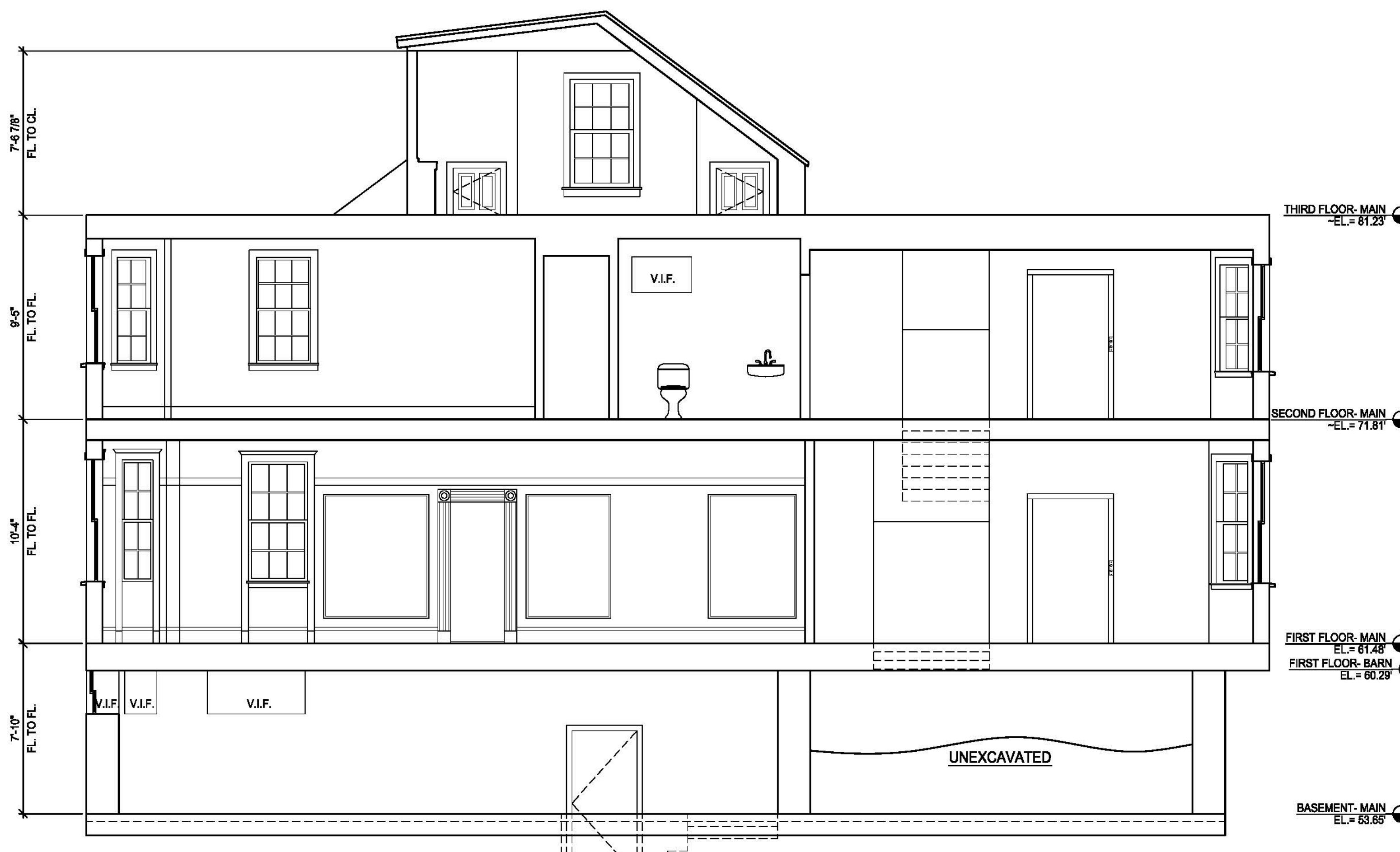
2 PROPOSED BUILDING SECTION A3.0 SCALE: 1/4" = 1'-0"
