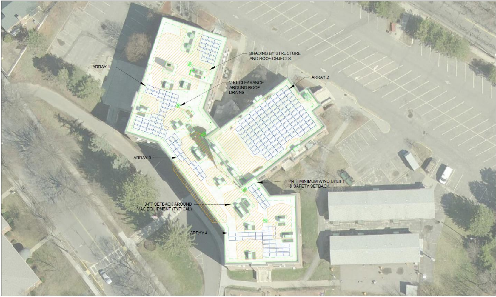
EDUCATION CENTER - OVERALL ARRAY LAYOUT SCALE: 1"=16' WHEN PRINTED 36" x 24"
