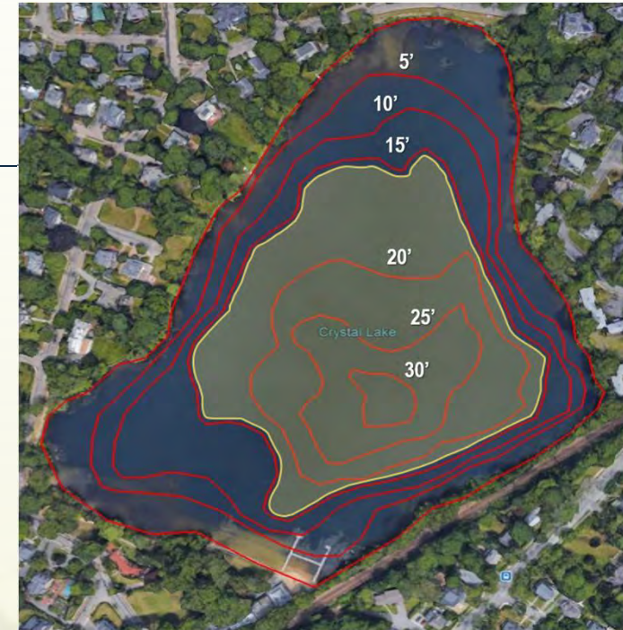
Crystal Lake Bathymetry and Approximate Nutrient Inactivation Control Area (in yellow)
