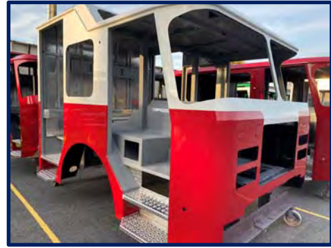
New Fire Engine #2 (in construction)
