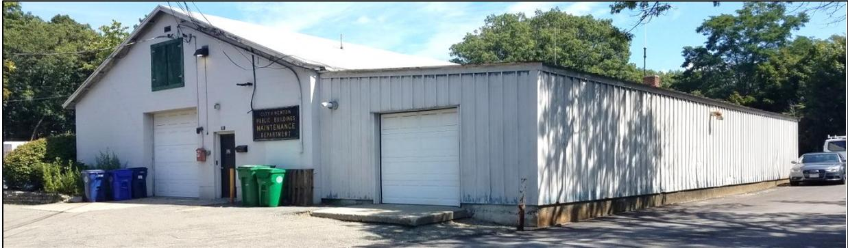
This building is 7,640 square feet. The building is comprised of a 3,780 square foot concrete block garage built in 1968, a 1,700 square foot metal prefab garage added in 1976, and a 2,160 square foot wood framed modular section added in 1980. This facility has 25 employees assigned to it, 12 of which have assigned offices that are heavily occupied. The other 13 employees are trades craftsmen who use the facility for work assignments and bathrooms.
