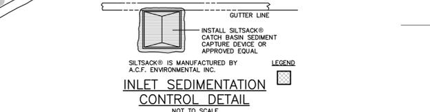
**INLET SEDIMENTATION CONTROL DETAIL**
