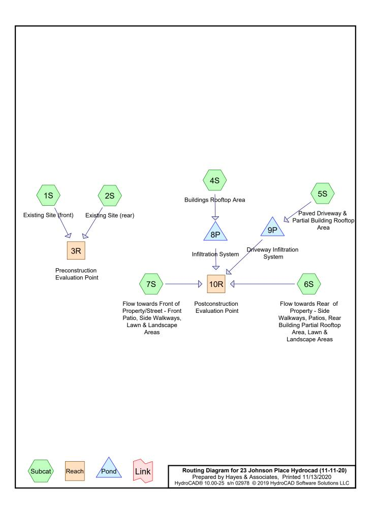
Prepared by Hayes & Associates HydroCAD® 10.00-25 s/n 02978 © 2019 HydroCAD Software Solutions LLC
