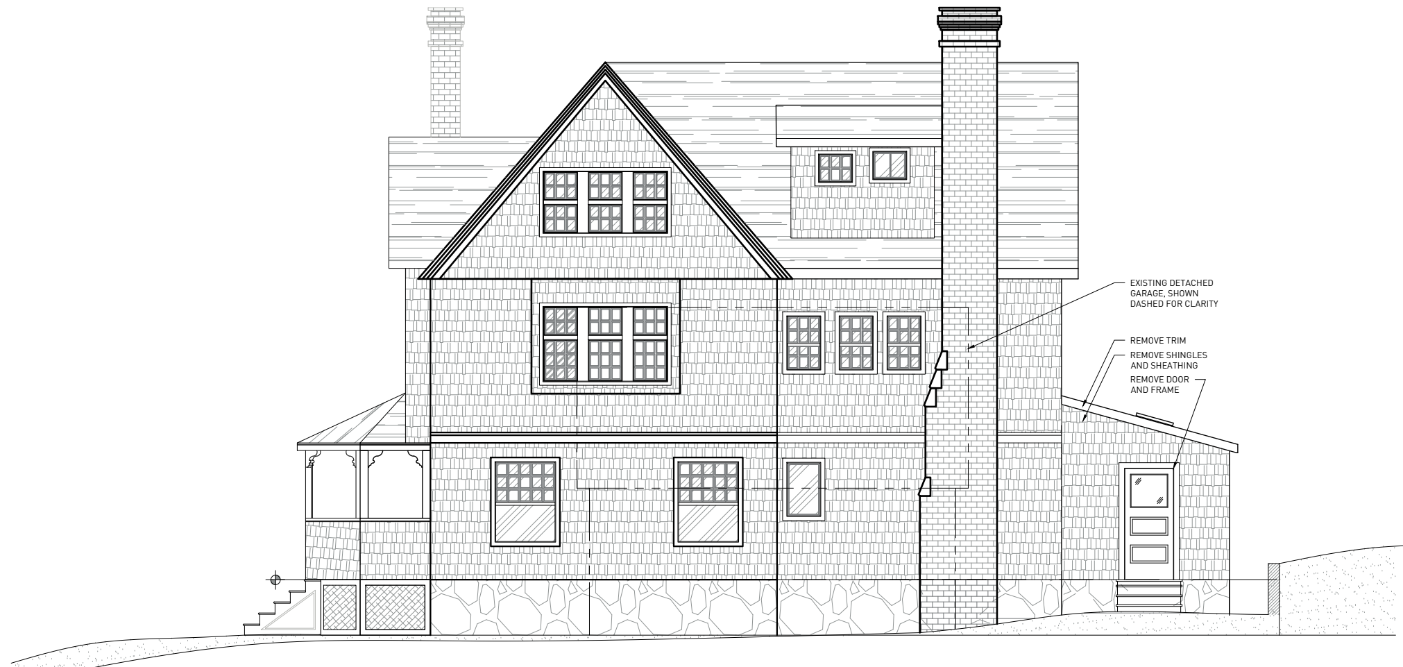
A NORTHEAST FACING ELEVATION - EXISTING / DEMO.
