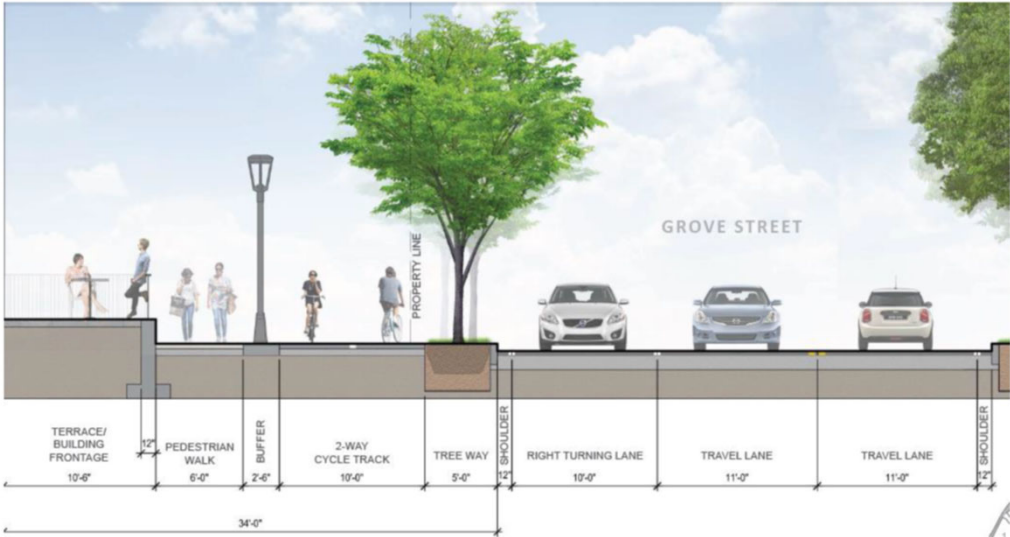
Grove Street section - 11' lanes, 10' turning lane, 1' shoulder.
