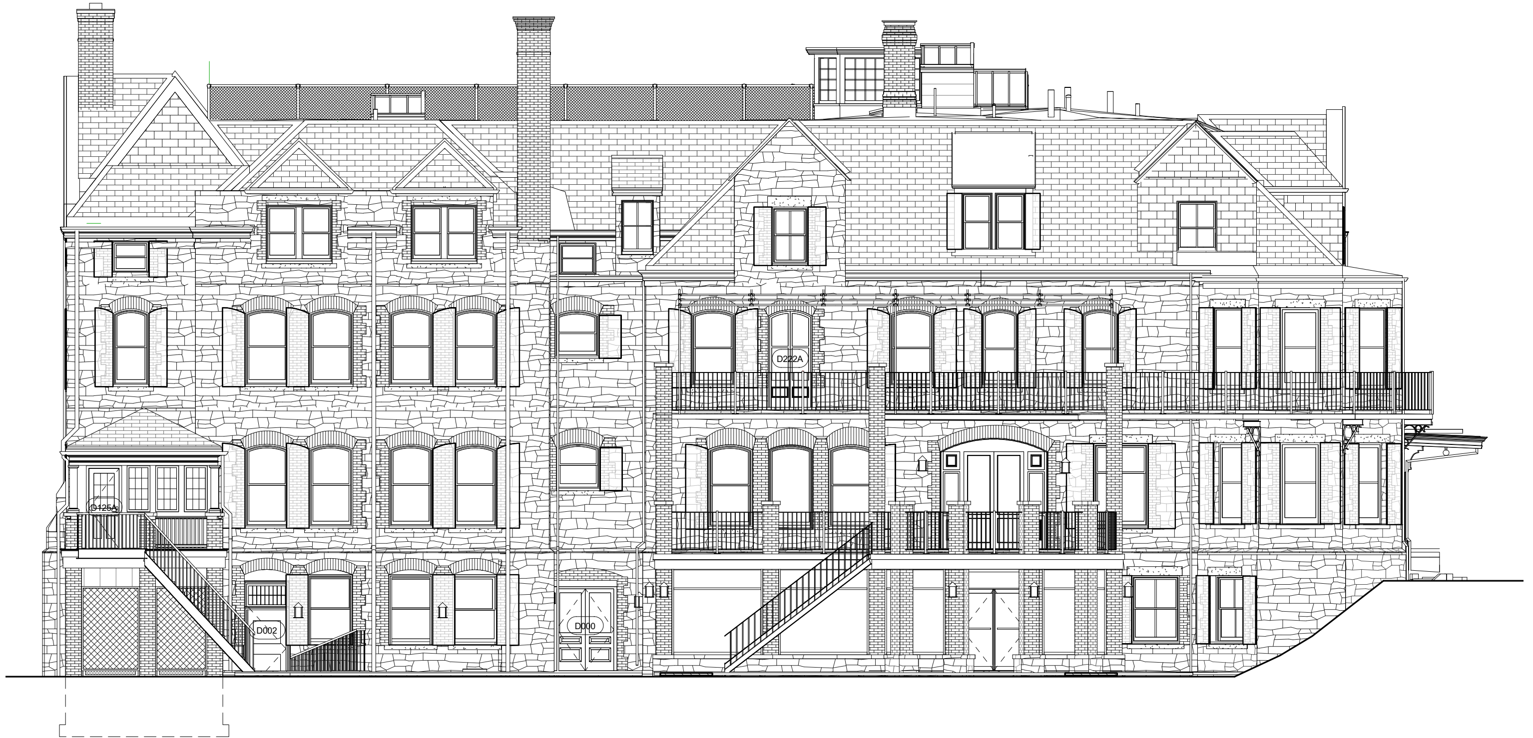
① SOUTH ELEVATION WITH PROPOSED NEW GUARDRAILS 1/8" = 1'-0"
