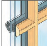
OGEE INTEGRAL LIGHT TECHNOLOGY 1 7/8", 1-1/4" OR 2"
