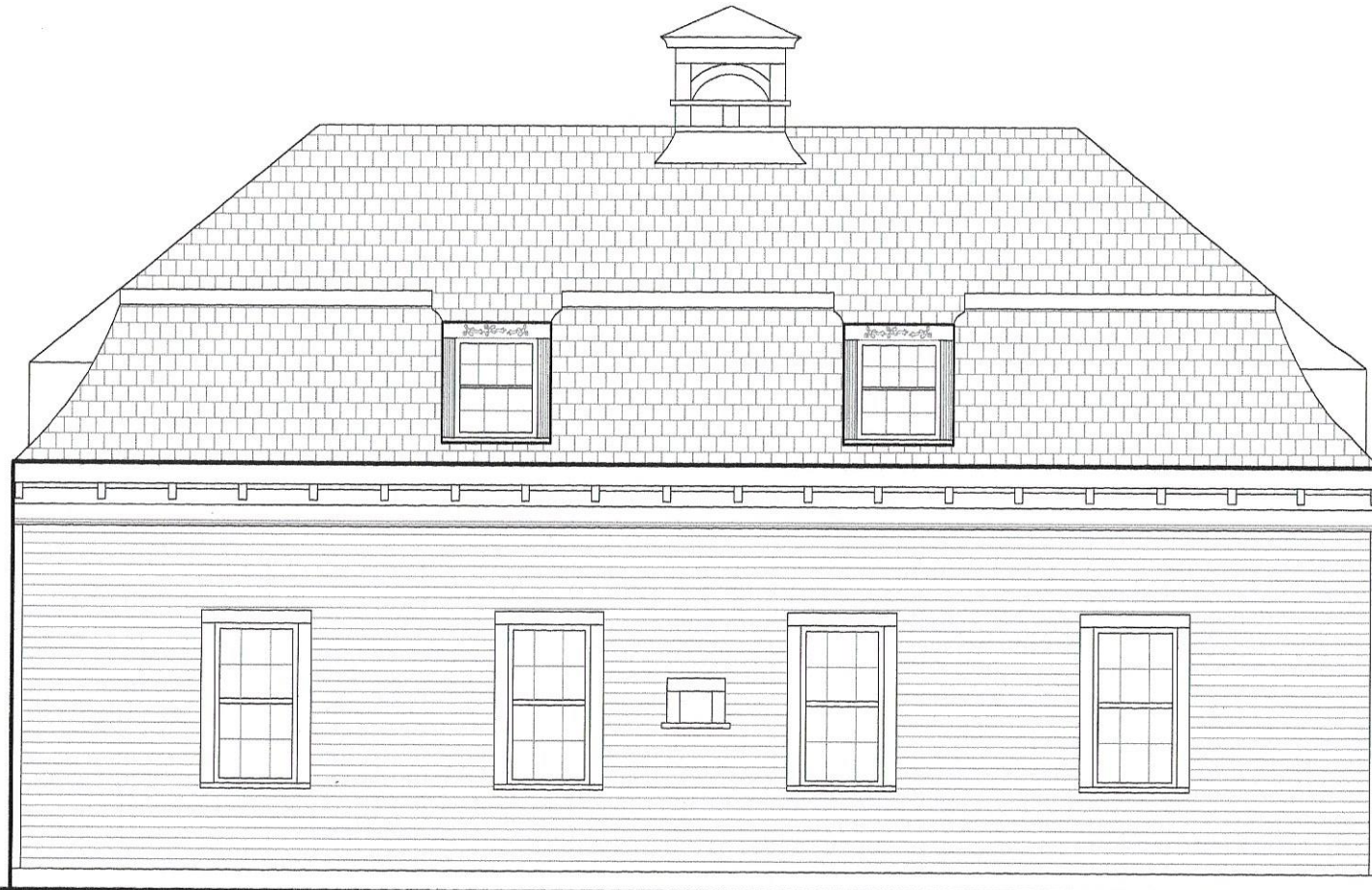
3 PROPOSED REAR ELEVATION SCALE: 1/4" = 1'-0"
