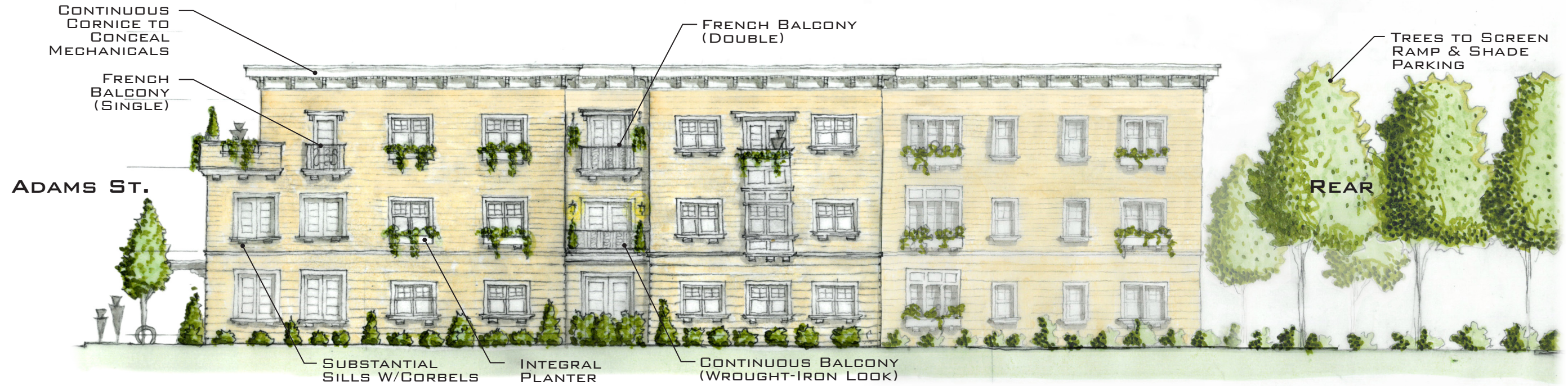
SIDE ELEVATION FACING DRIVEWAY
