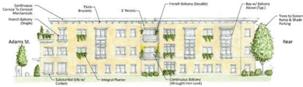
Side Elevation Facing Driveway
