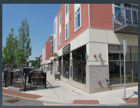
Cement Board may be appropriate for Austin Street but not on the ground floor, close to pedestrians, as was done in the developer's project in Reading.
