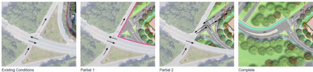
Figure 1044 – Grove Street/Recreation Road Traffic Maintenance
