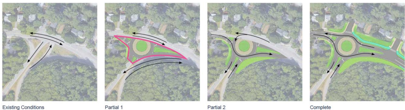
Figure 1140 – 128 South Roundabout Traffic Maintenance
