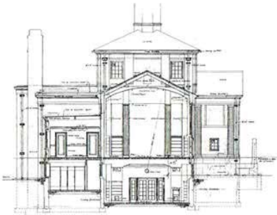
The original cross section drawing of the Library showing the raised main floor level 5 feet above outside grade
