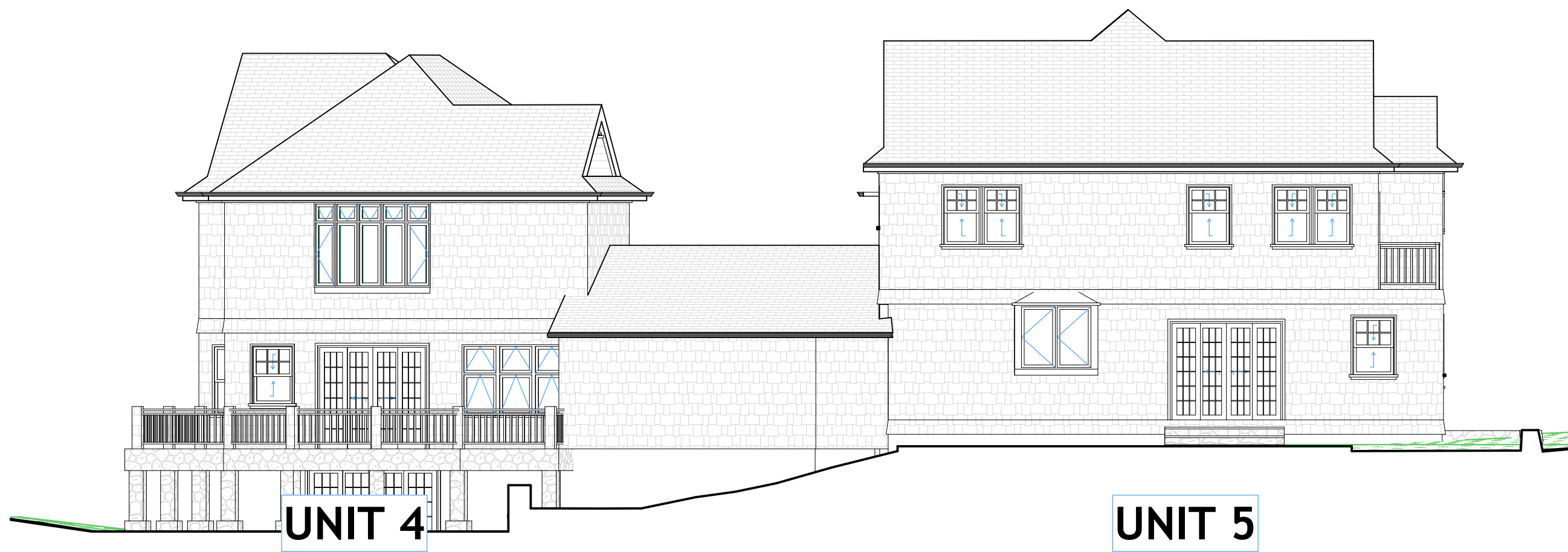
A-201 NORTH ELEVATION (SIDE) 1/8" = 1'-0"
