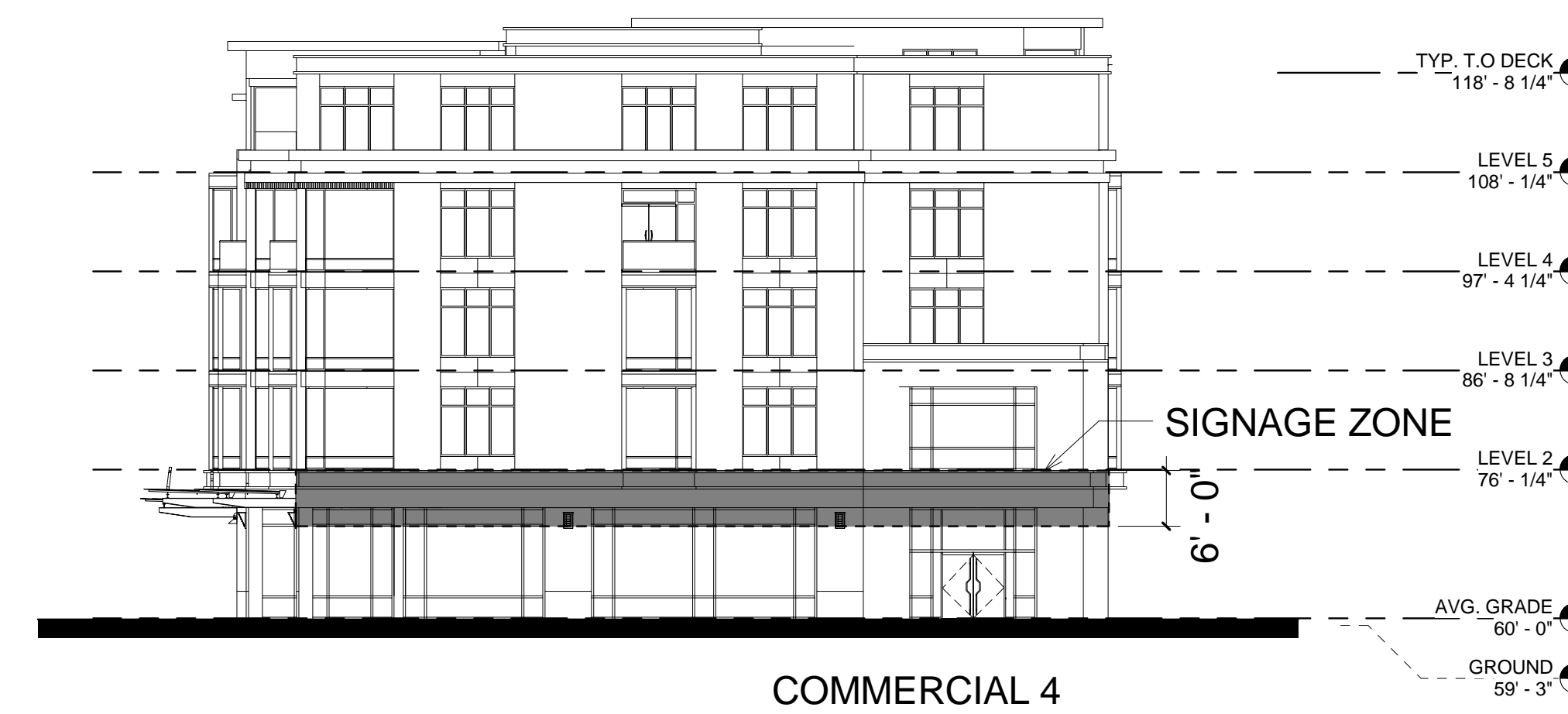
4 COURTYARD ELEVATION 3 - SIGNAGE 1/16" = 1'-0"
